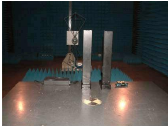
7.6. Photo of EFT/surge/Dips immunity measurement (E.F.T./Surge./Dips.)
