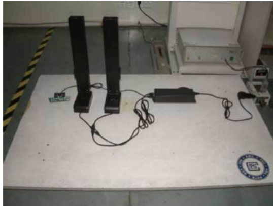
7.7. Photo of conducted disturbance Immunity measurement (C.S.)
