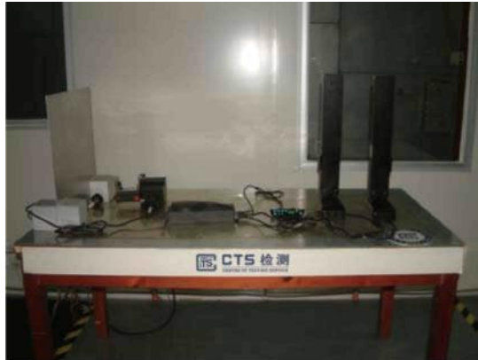
7.4. Photo of electrostatic discharge Immunity measurement (E.S.D.)
