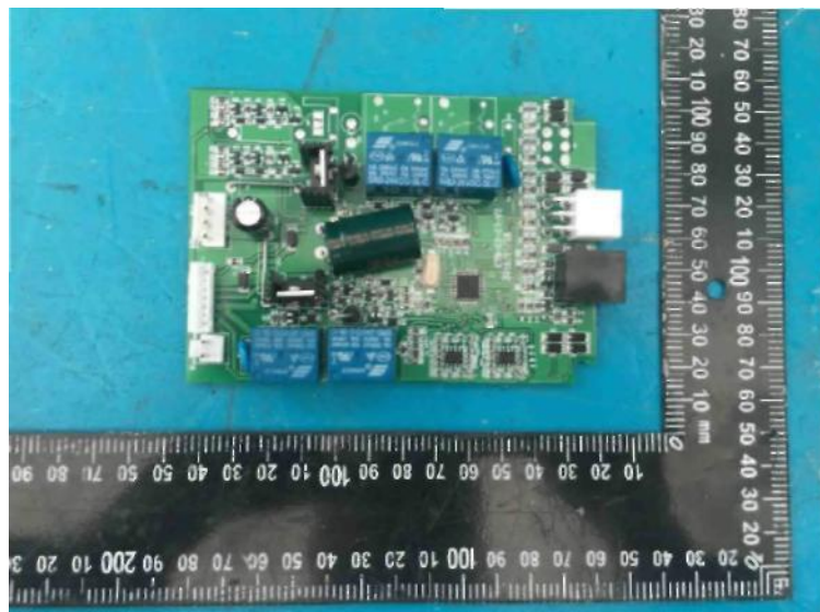
Fig.8 - Top view of Control Board
